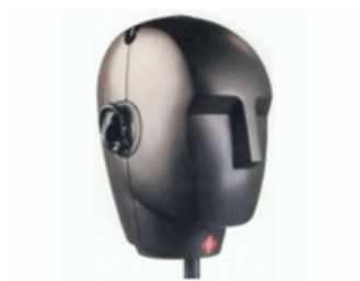
An artificial head with microphones mounted into the ears
