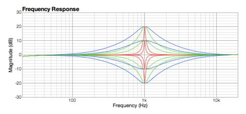
Figure 19: EQ peak and notch filters
