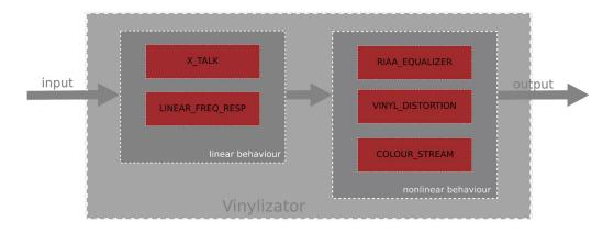
Figure 25: Block diagramm of the Weiss Vinyl Emulator
