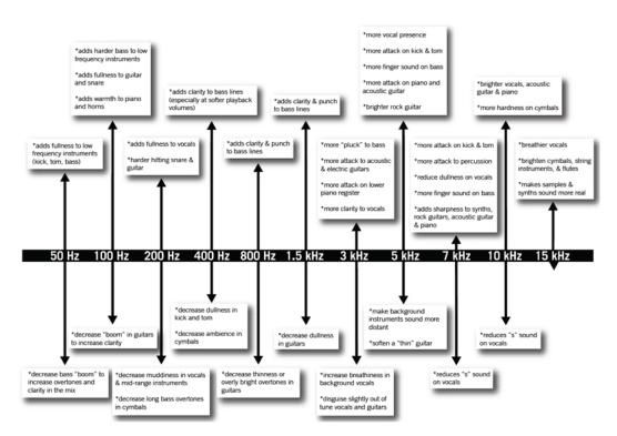
Figure 22: Instruments' spectral treatment overview
