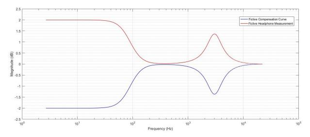
Figure 34: Fictive example of a headphone frequency response measurement (red) and its correlated compensation curve (blue).
