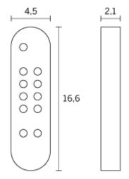
Figure 18: Engineering drawing of IR remote control
