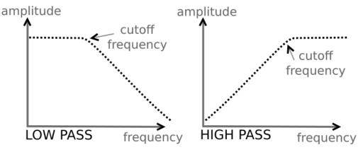
Figure 21: Low pass and high pass filter scheme
